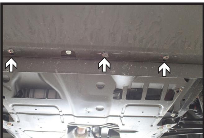
5. Using a T30 Torx, remove the three (3) screws from the underside of the fascia. **DO NOT** remove the silver screw.
