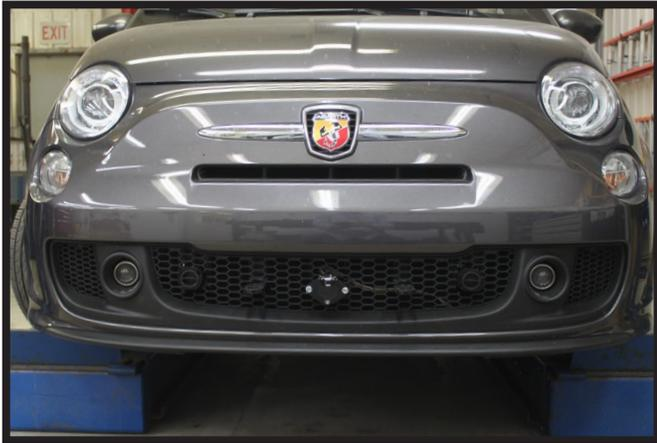
10. Hold the fascia up to the vehicle as close to it's original position. Mark and trim with a utility knife until the fascia is clear of the attachment tabs and convenience links.
