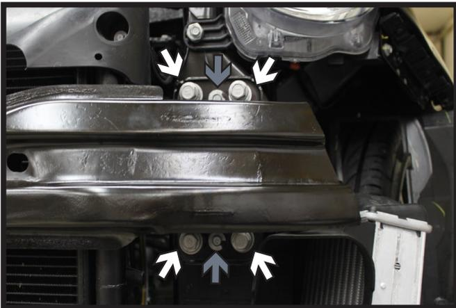
7. Using a 15MM socket, remove the four (4) larger bolts from bumper (white). Then using a 10MM socket, remove the two (2) smaller bolts (gray). Repeat on the other side of the vehicle. The metal bumper and smaller bolts will not be reused.
