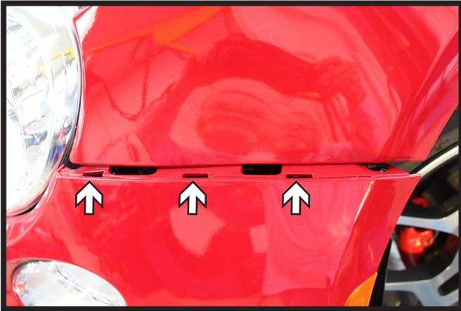
6. Unsnap the fascia from each side. Unplug all electrical connections, then pull fascia outwards to remove from the vehicle.
