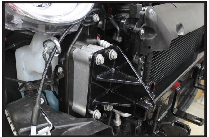
8. Install the baseplate onto the vehicle, using the existing spacer and 10MM bolts. Repeat on the other side of the vehicle. Tighten down baseplate to the vehicle.
