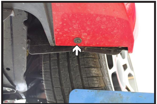
4. Using a phillips screwdriver, remove the one (1) screw from the underside bottom corner of the fascia. Repeat on the other side of the vehicle.
